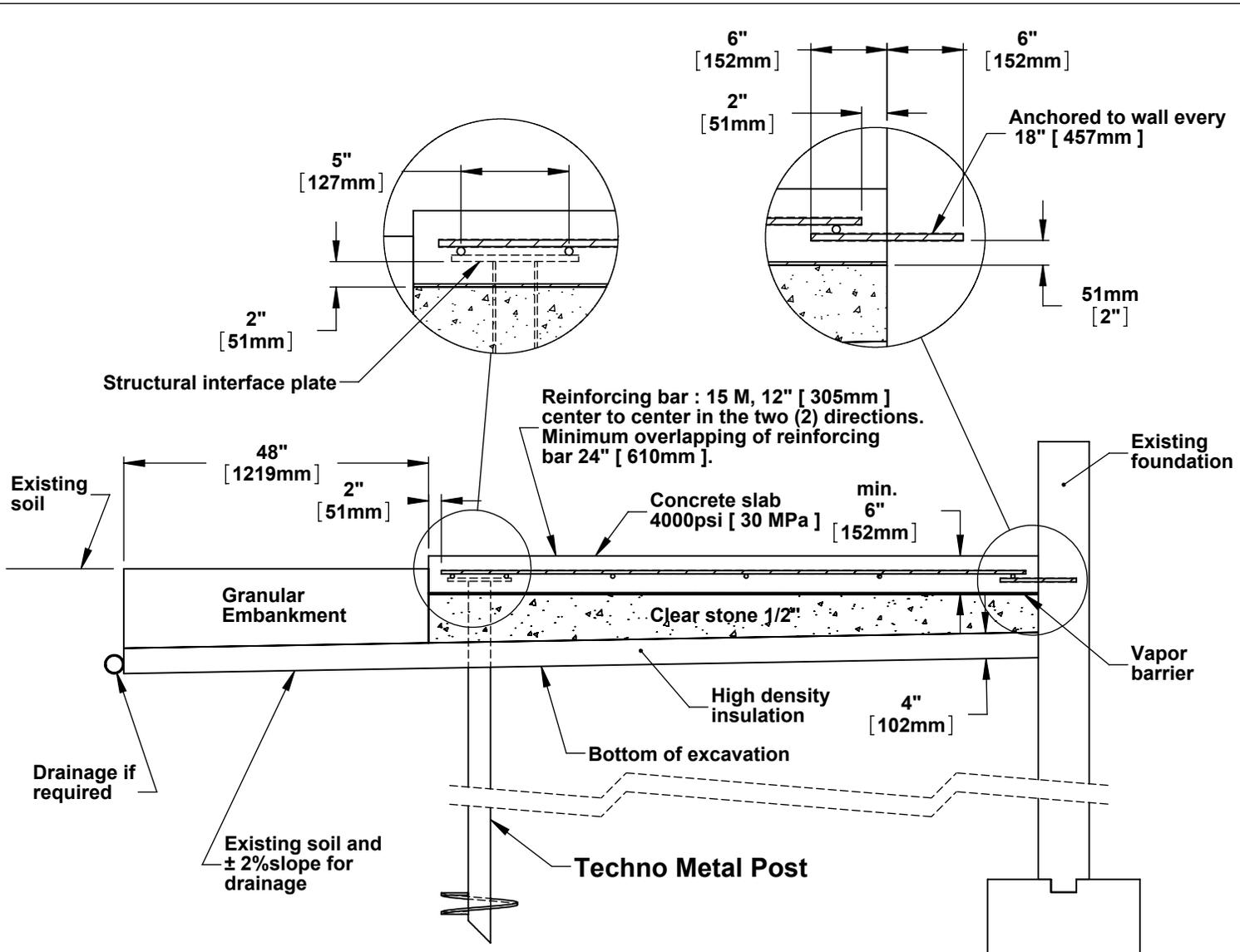
**Note :** Be aware that it is your responsibility to adequately protect the concrete slab on ground against freezing and it is important to drain the concrete slab, in order to avoid any movement of rising ( concrete slab and the Techno Metal Post ) during the period of freezing-thawing winter.
